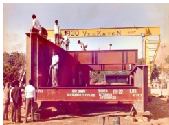
500MW – TALCHER BOILER -0617 CEILING GRIDER'C WEIGHT ABOUT 78,273 kgs FABRICATED BY M/s.VKN INDUSTRIES (BO1) UNDER STRINGENT QUALITY CONTROL cleared by QC/BHEL and NTPC , delivered on 16-11-2000 to M/s.BHEL ,Trichy.
