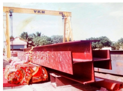
PLUS – TYPE COLUMN fabricated by M/s.VKN INDUSTRIES for M/s. BHEL.
