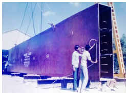
BOX GRIDER fabricated by M/s.VKN INDUSTRIES for NEYVELI PROJECT
