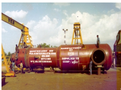
37648Kgs of GASSIFIER ASSEMBLY Fabricated by M/s.VKN Industries Cleared by QC/BHEL under Stringent Quality control Dispatched to
