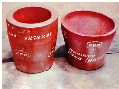
PRESSING OF REDUCER pressed by M/s VKN INDUSTRIES in 1000 TON HYDRAULIC PRESS.
