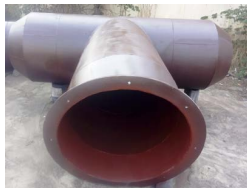
TEE- Duct fabricated by M/s.VKN INDUSTRIES
