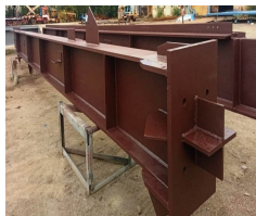
Build-Up section Fabricated by M/s.VKN Industries
