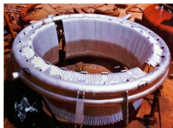
SKIRT ASSEMBLY for ROURKELA STEEL PLANT fabricated by M/s.VKN Industries.
